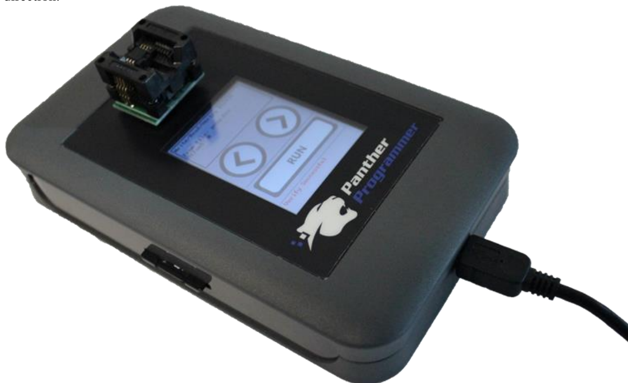
SO-8 Memory Device Setup
